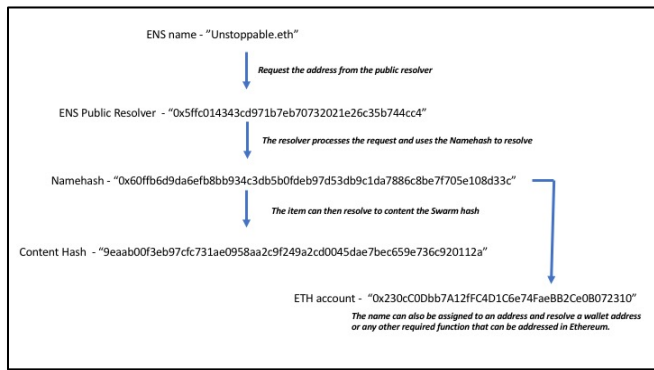
Figure 3. A breakdown of the ENS and the different elements involved in name resolution
